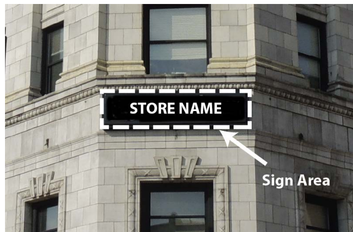
Figure 1281-3: Illustration of computing the sign area for wall signs with a background panel or cabinet.
