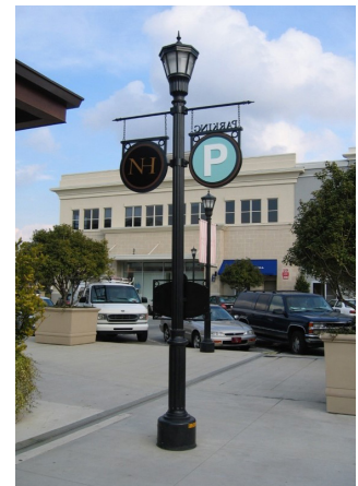
Pedestrian-scale lighting. Cut-off style fixtures reduce glare and light pollution.
