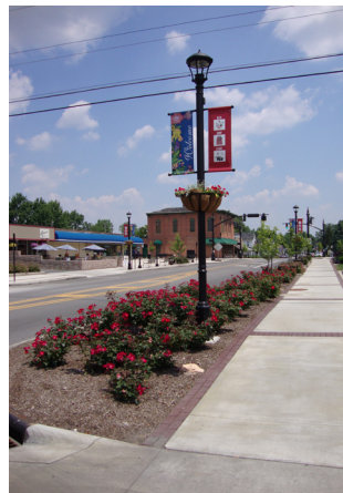
Pedestrian-scale lighting. Cut-off style fixtures reduce glare and light pollution.
