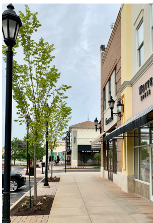
Sidewalks along a high volume street with parking spaces should allow for street trees and/or landscape beds at intervals for optimal pedestrian access.
