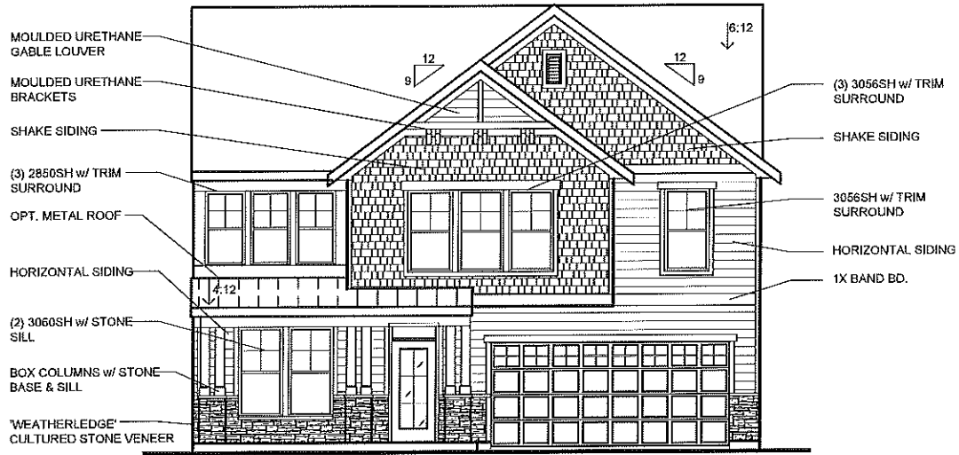
INC. FRONT ENTRY w/ INC. SIDING
