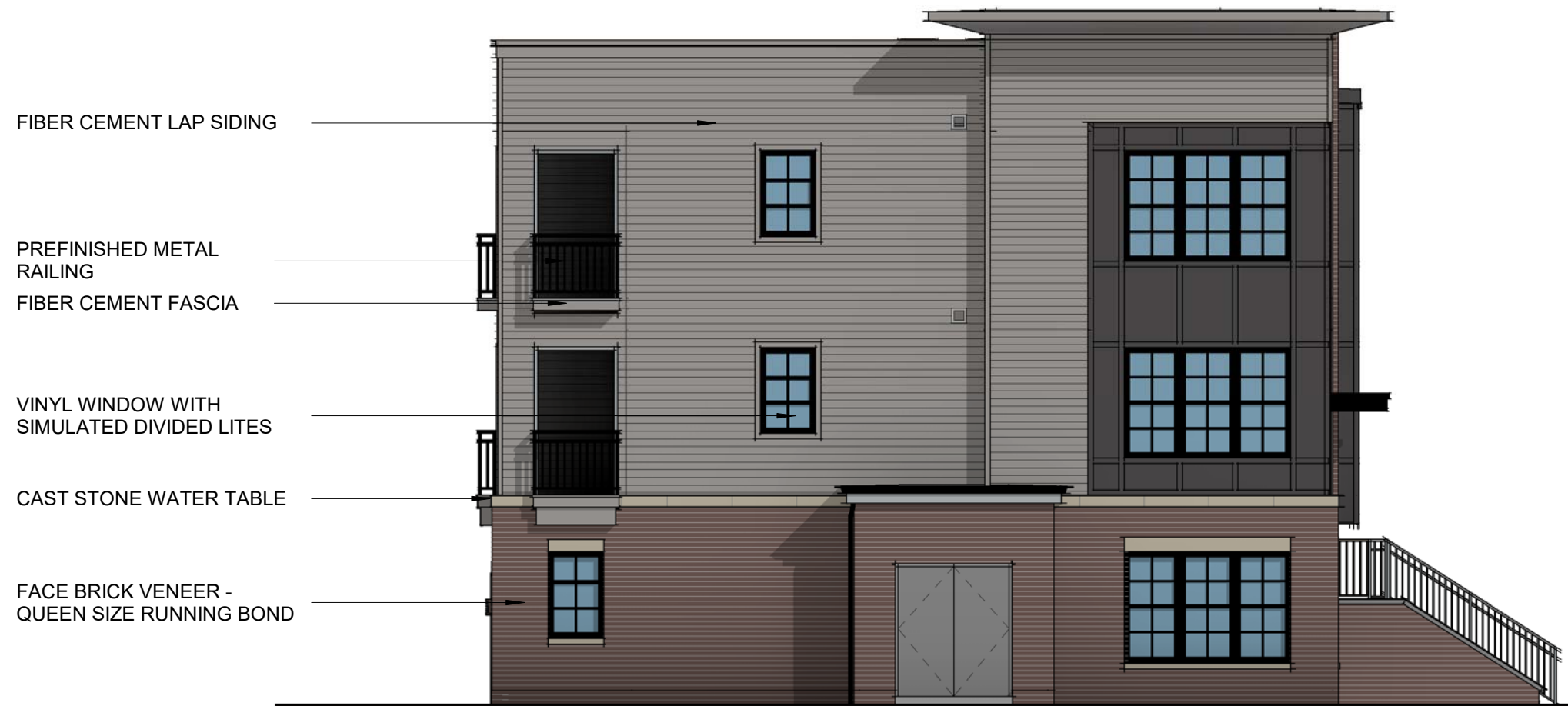
Building Type E - Side Elevation 1/8" = 1'-0"
