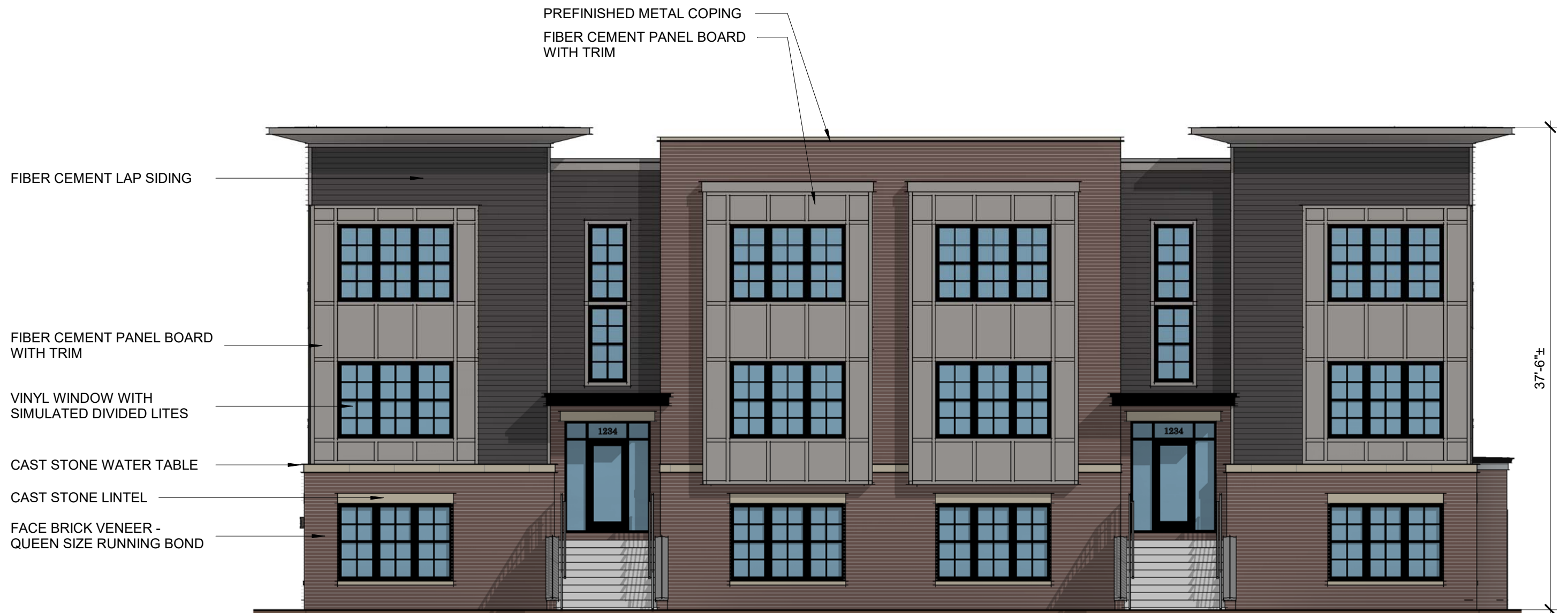
Building Type D - Front Elevation
